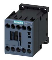
Power contactor, AC-3 12 A, 5.5 kW / 400 V 2 NO + 2 NC 24 V DC 4-pole Size S00 screw terminals
